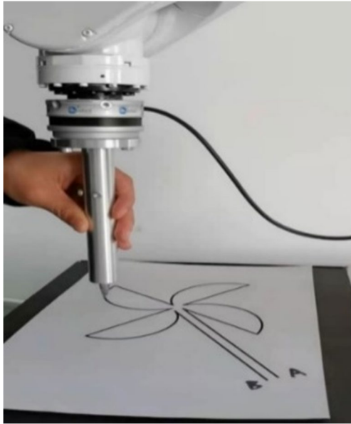
Fig. 1 Human guiding a robot for drawing a complex pattern
