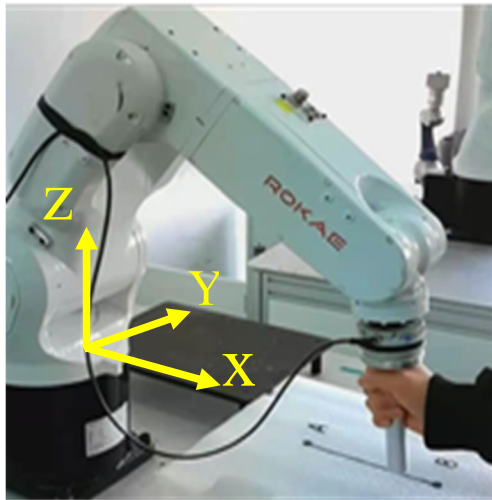
Fig. 7 Human guiding for a robot’s linear motion
