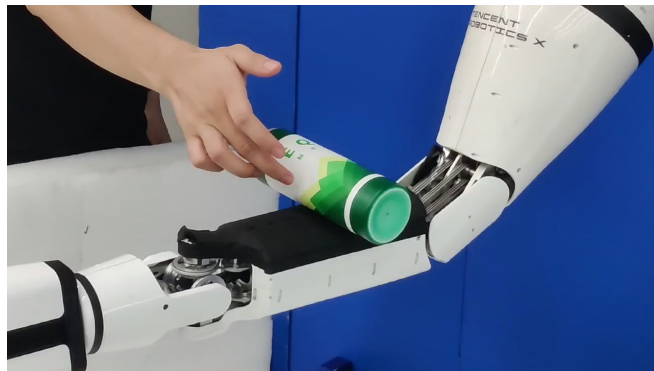
Fig. 1. Stability regulation of a bottle positioned on a robotic arm subject to manual disturbances. Tactile servoing is performed on a custom tactile sensor array covered by black foam on the forearm.
