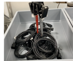
Fig. 9. Grasping unseen cable from clutter.
